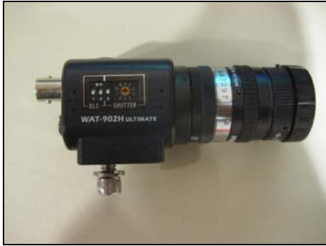
Foto 3 : de WATEC 902H-ultimate in detail
