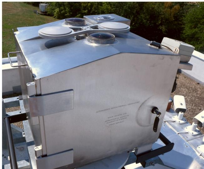
**Fig. 1.** Digital Autonomous Fireball Observatory (DAFO) with the lens cover open at its site in Ondřejov. The Aurora weather sensor is on the right, next to the GPS receiver. The radiometer window is at the back right corner.
